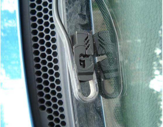
Insert plastic clip part way into "U" form of wiper arm, taking care not to push slot too far, so the bottom part of "U" form doesn't cover it.(see 2 pics above)
