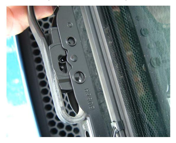
With clip in position, offer the Bosch wiper blade underneath.so pin in wiper will line up with slot in plastic clip. (pic above)
