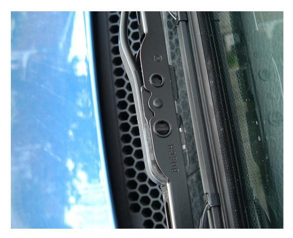
Push plastic clip and wiper arm into blade until pin clicks into position of plastic clip.
